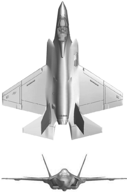
Fig. 1 Sketch of the 1/15th-scale baseline CV model of the JSF. S_{\text{ref}} = 2.76 \text{ ft}^2 , b_{\text{ref}} = 2.87 \text{ ft} , and c_{\text{ref}} = 1.113 \text{ ft} .
